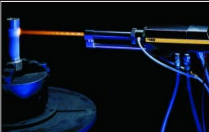
*The JP-5000 High Pressure HVOF system sprays with the highest velocities of any HVOF system. This improves coating quality density and bond strength.*
